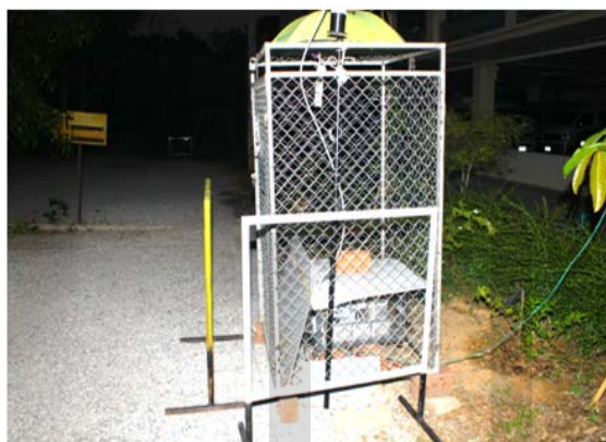
Figure 1. Gent Air Sampler at sampling site for collecting PM 10
